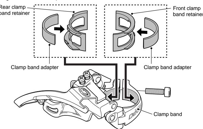
**Note:** The clamp band adapters and the front and rear clamp band retainers are all available in two sizes: S size (28.6 mm diameter) and M size (31.8 mm diameter).
